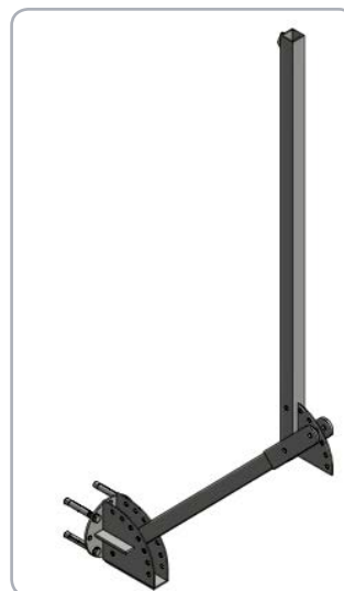
Fixation with 4 M14 expanding anchors.
